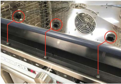
On the lower part of the control panel, loosen and remove the two black mounting knobs.
