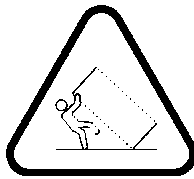
TIP AND CRUSH HAZARD
