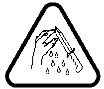
SHARP MACHINE PARTS HAZARD
